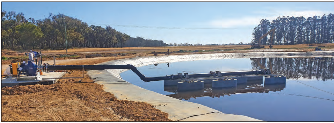
The Gorman-Rupp 86B3 self-priming pump securely mounted on the lagoon bank eliminates the need for workers to enter or operate directly on the water.
