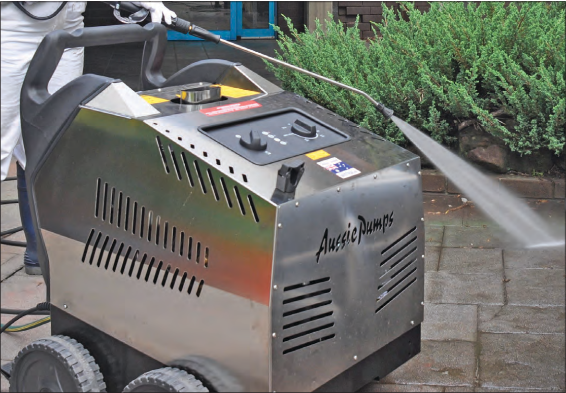
The Aussie Sizzler delivers 80C at 1800PSI. Used with a turbo, it's effective working pressure is 3100PSI. All this from a 240V 2.7kW single-phase motor.
