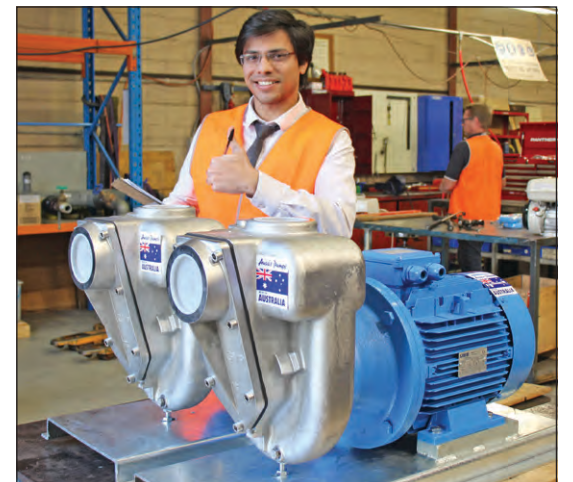
Aussie GMP motor pump with new 316 stainless steel is corrosion and abrasion resistant.
