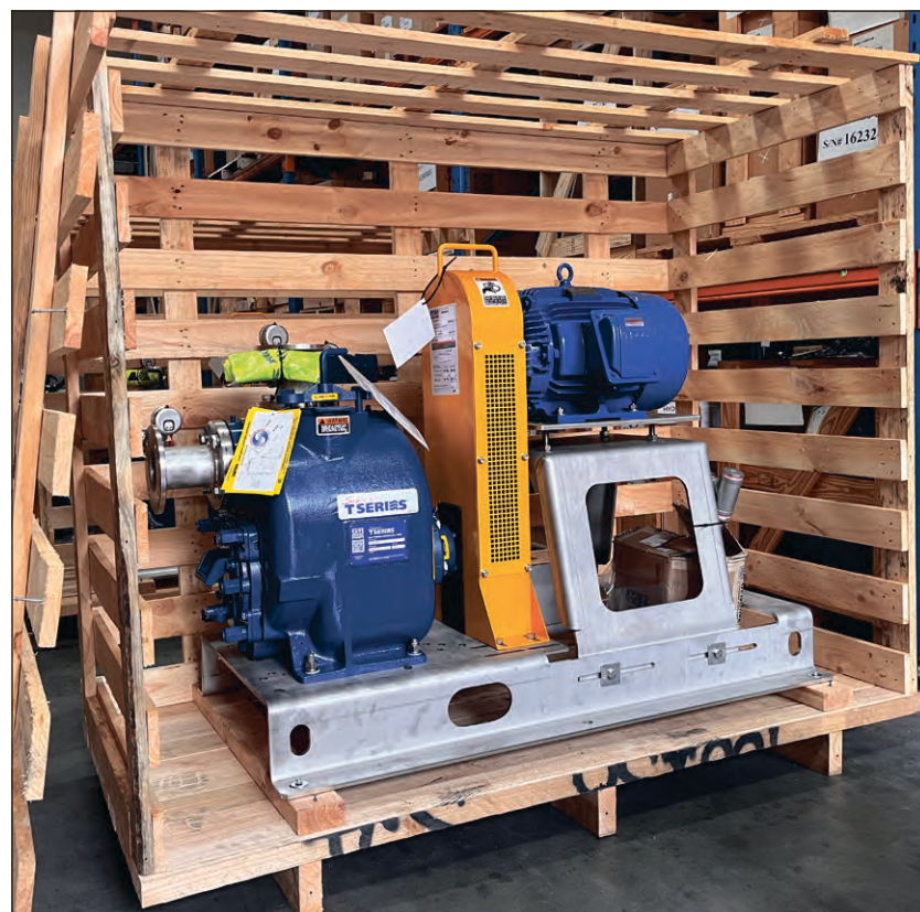
A Gorman-Rupp T3A71S-B pump with hardened internals was selected for the harsh environment of the refinery's recovery pit.
