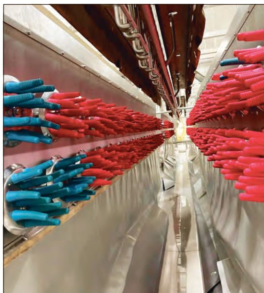
Duram's colour options make it easy to identify replaced fingers and differentiate machine setups.
