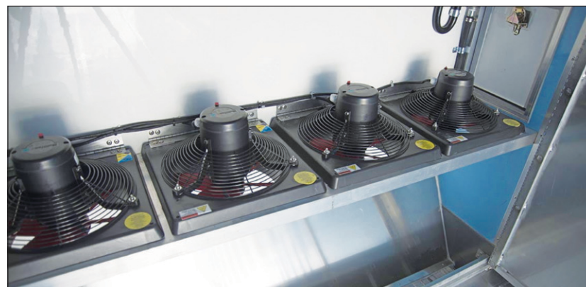
Powerful air management systems distribute controlled air within the load space, without upsetting the cargo.
