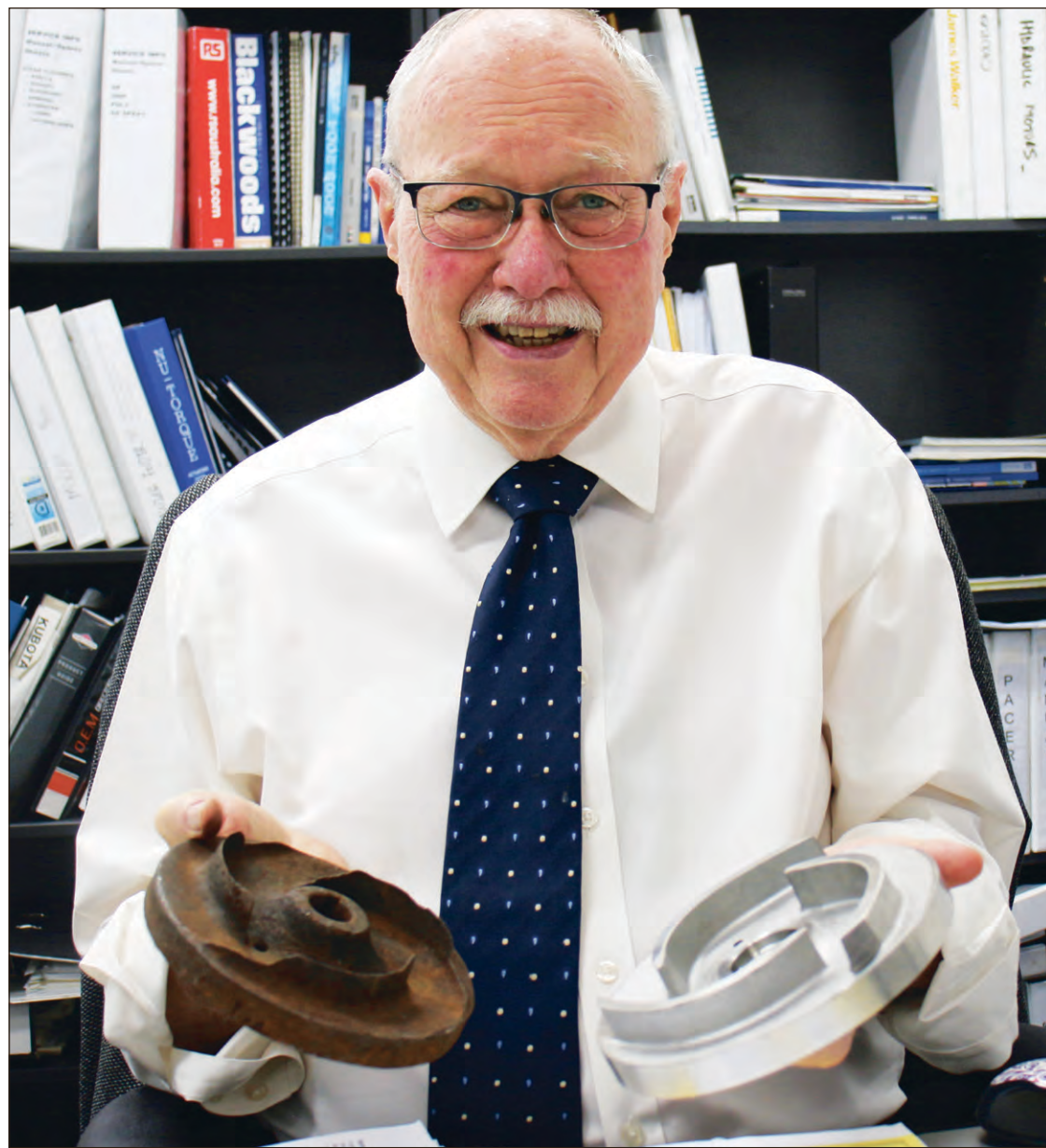
John Hales shows how cast-iron impellers erode in corrosive applications.
